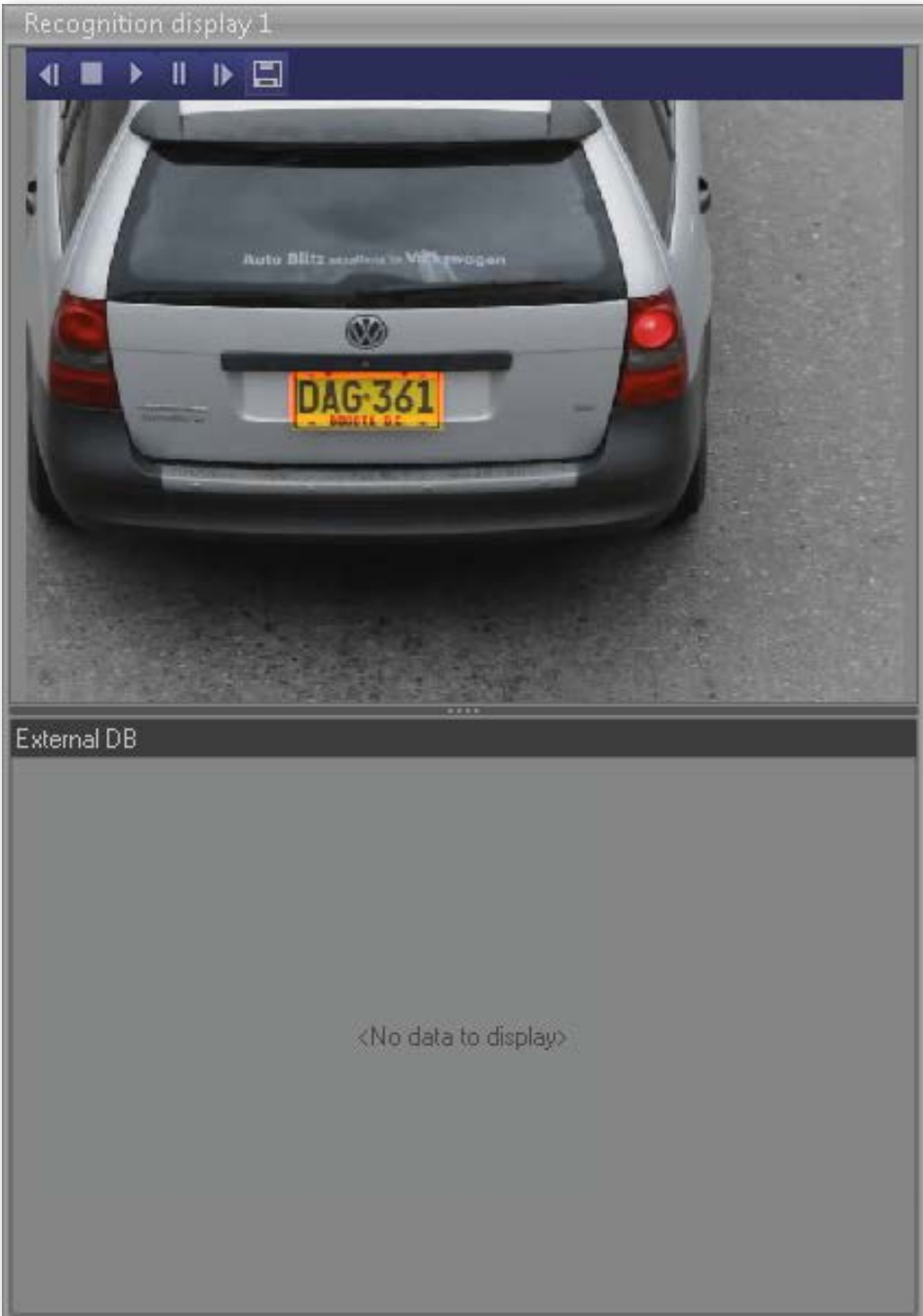
Figure 8 — Displaying the frame with last recognized license plate in Recognition display window
