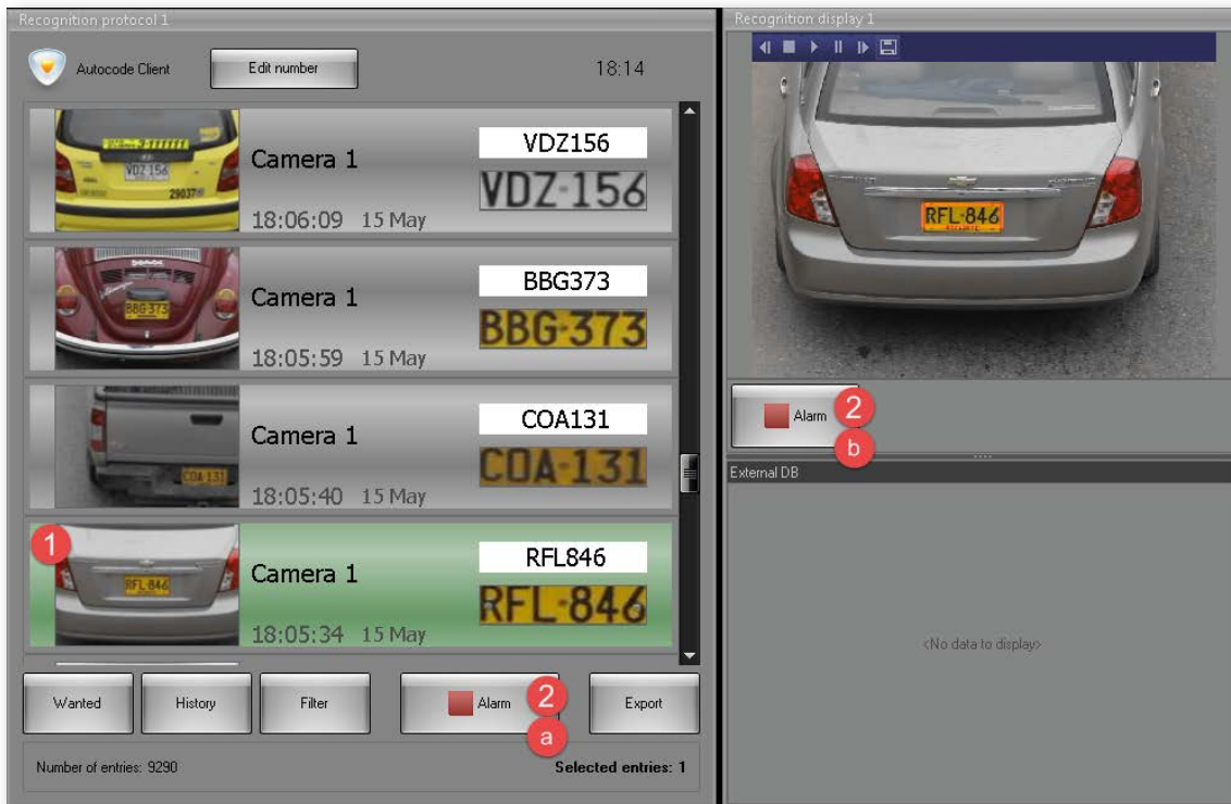
Figure 13 — Initiating alarm manually
