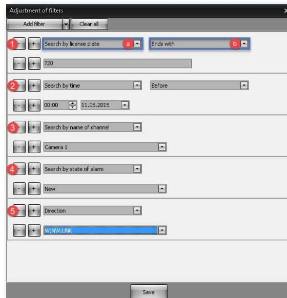
Figure 5 — Adjustment of filters window: available filters and filtering criteria
