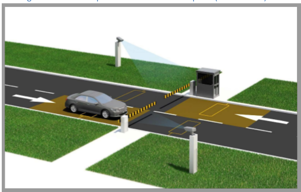
Figure 10 – Camera placement on the access point (barrier used)
