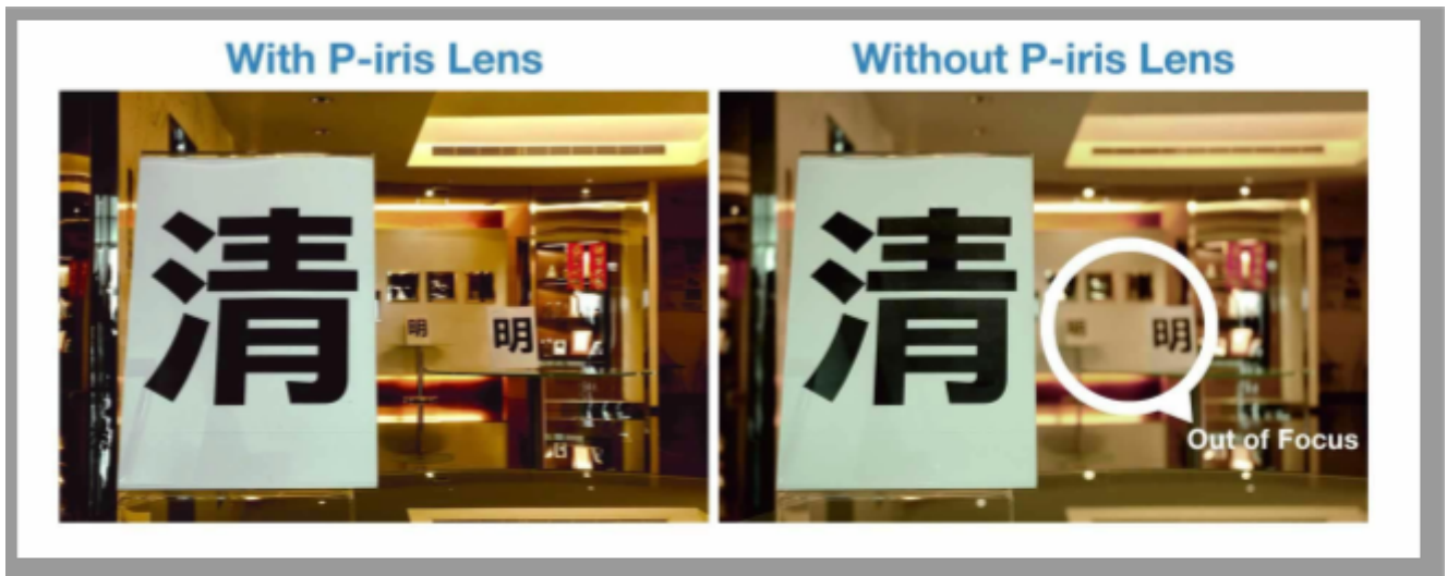
Figure 4 – Comparing sharpness of images taken with and without P-iris
