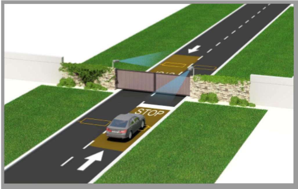
Figure 11 – Camera placement on the access point (a solid obstacle is used)
